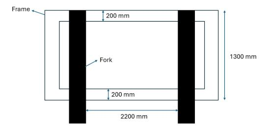
Determine the profile shape function, f(x), also the thickness of the vertical section, all assuming infinite life safety factor of 1.5. The vertical section of the forks has a uniform section.
