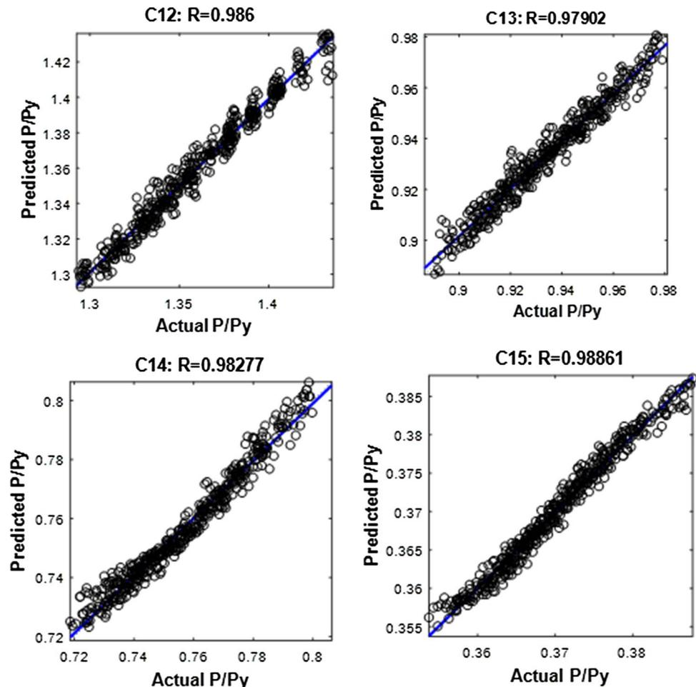
**Fig. 9** Comparison of the actual values calculated from the finite element analysis and the values predicted by ANN for the ratio  $P/P_y$  of columns in removal of the interior column  $C_{12}$
