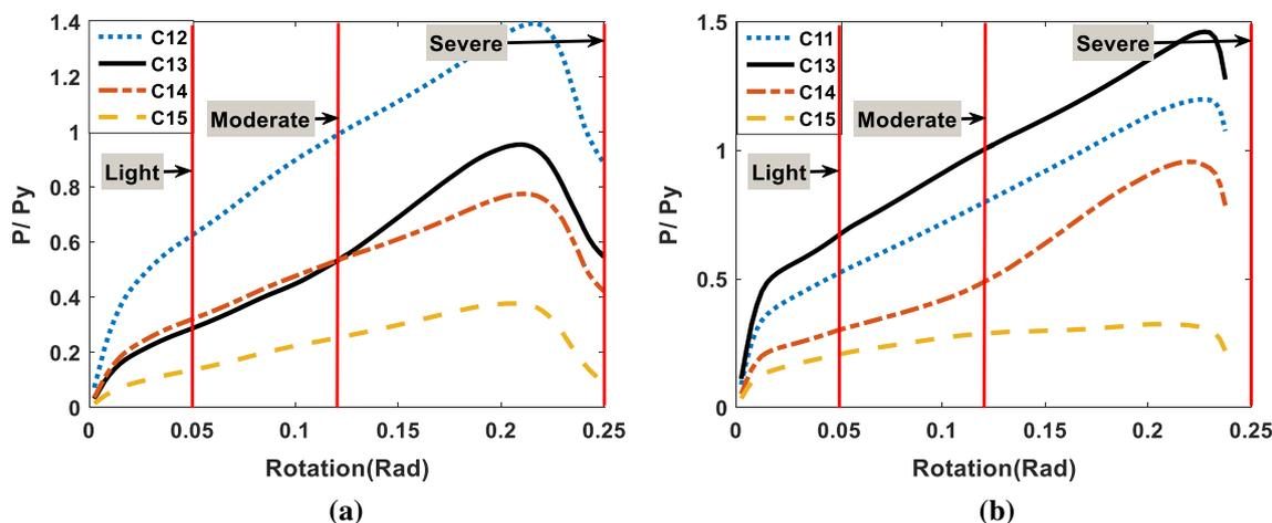
Fig. 6 The ratio  $P/P_y$  for columns with considering catenary action: a the removal of the exterior column  $C_{11}$ ; b the removal of the interior column  $C_{12}$
