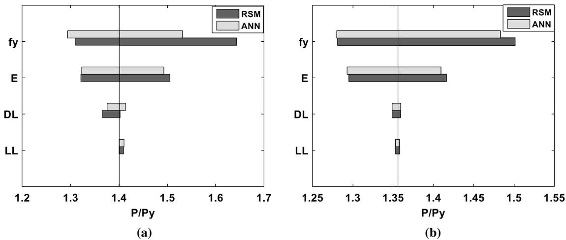
**Fig. 14** Tornado diagram derived from the sensitivity analysis based on ANN and RSM methods: **a** column  $C_{13}$  in the removal of the interior column; **b** column  $C_{12}$  in the removal of the exterior column
