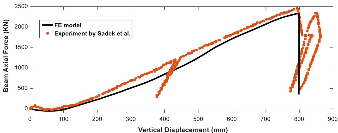
**Fig. 3** Comparison of the axial forces induced in the beam obtained from the analytical and the experimental results
