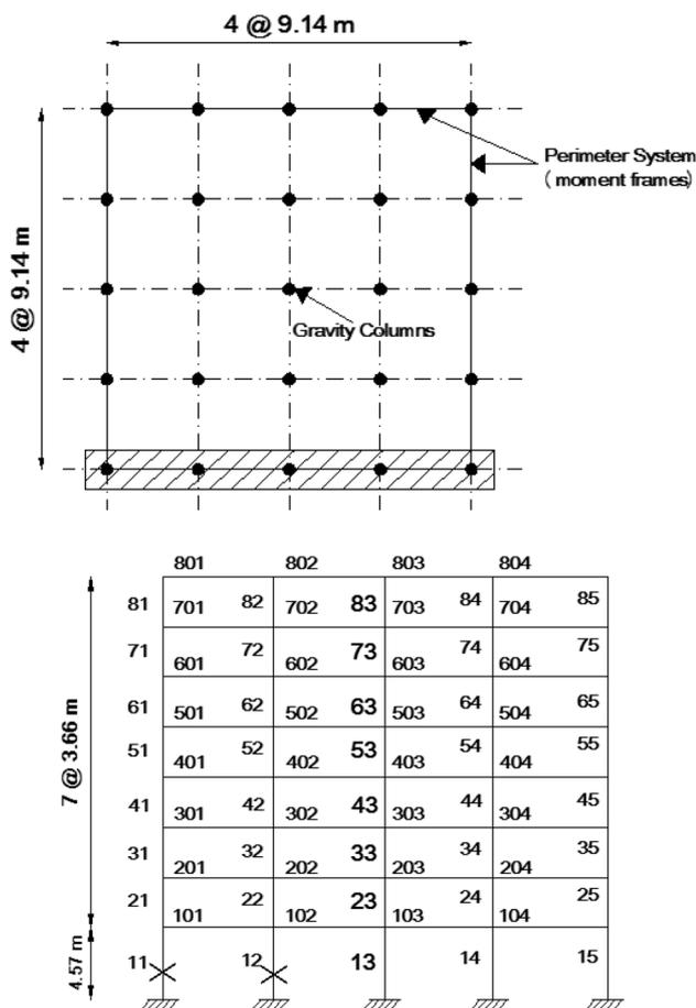
Fig. 4 Plan and elevation view of the structural model with scenarios of the column removal
