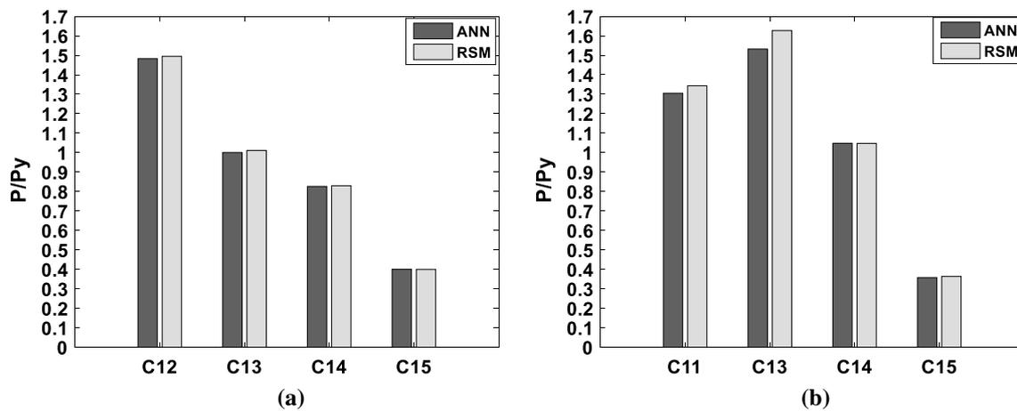
Fig. 13 Maximum ratio  $P/P_y$  of columns with  $10^6$  samples: **a** the removal of the exterior column  $C_{11}$ ; **b** the removal of the interior column  $C_{12}$
