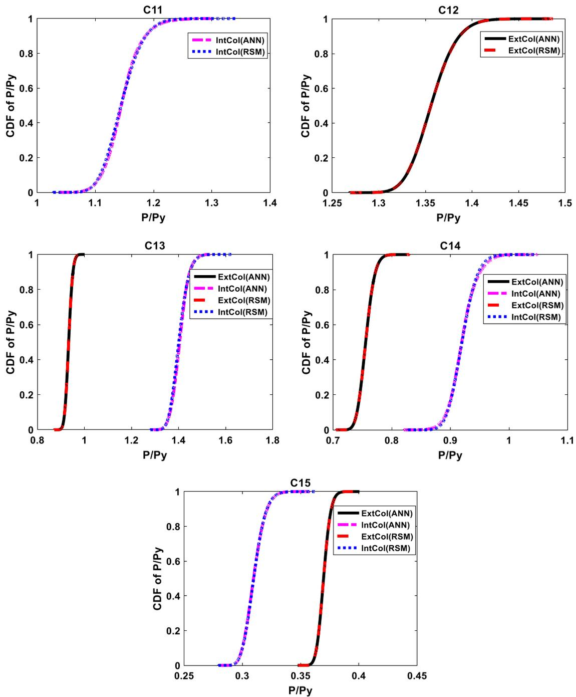
Fig. 12 Comparison of the cumulative distribution functions of the ratio  $P/P_y$  of columns in both column removal scenarios using RSM and ANN methods
