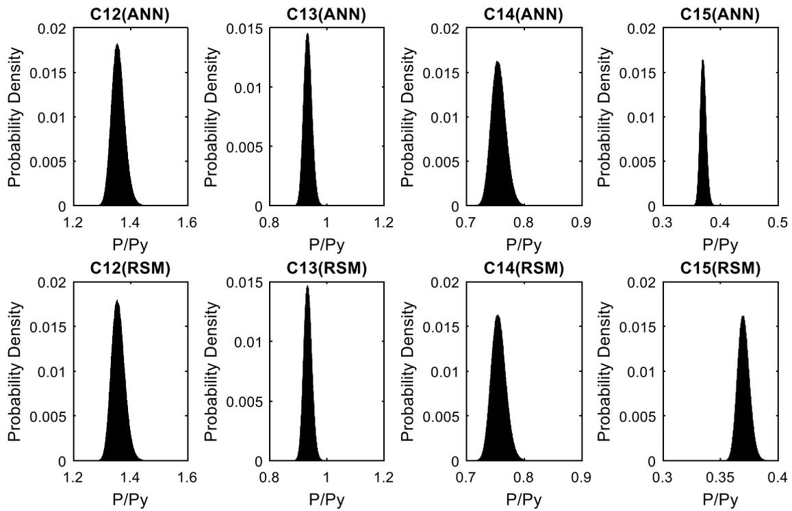
Fig. 10 Probability distribution for ratio  $P/P_y$  of columns using RSM and ANN methods under exterior column removal
