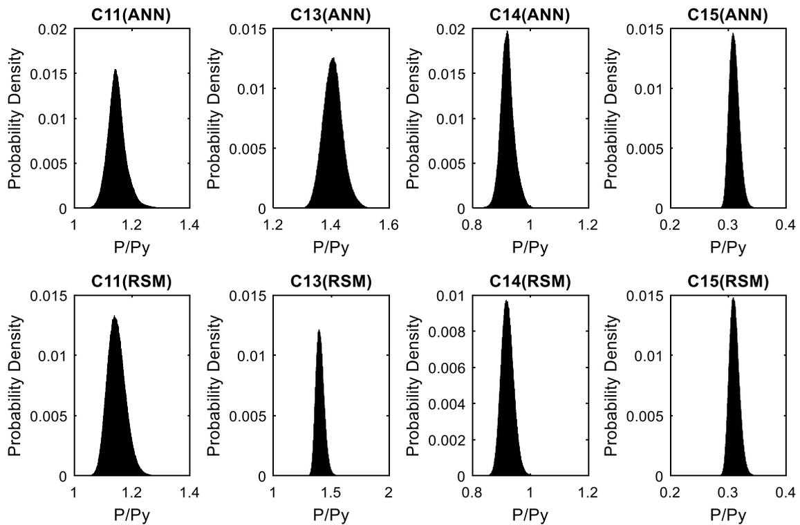
Fig. 11 Probability distribution for ratio  $P/P_y$  of columns using RSM and ANN methods under interior column removal
