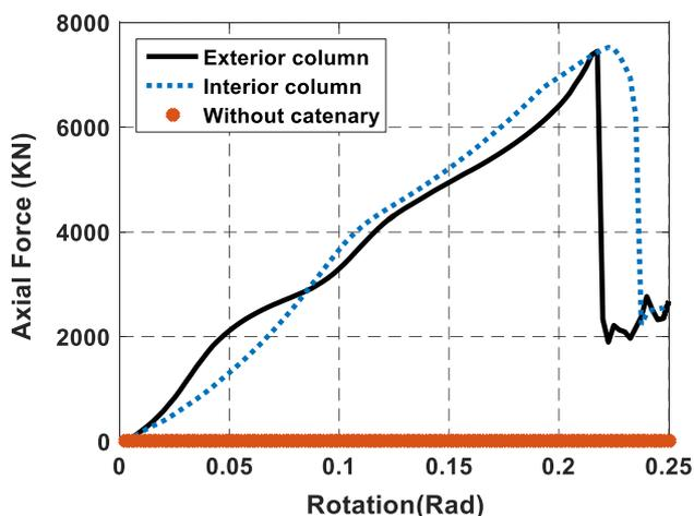
Fig. 5 Comparison of the axial forces created in the beam after the removal of the exterior and interior columns with and without considering catenary action
