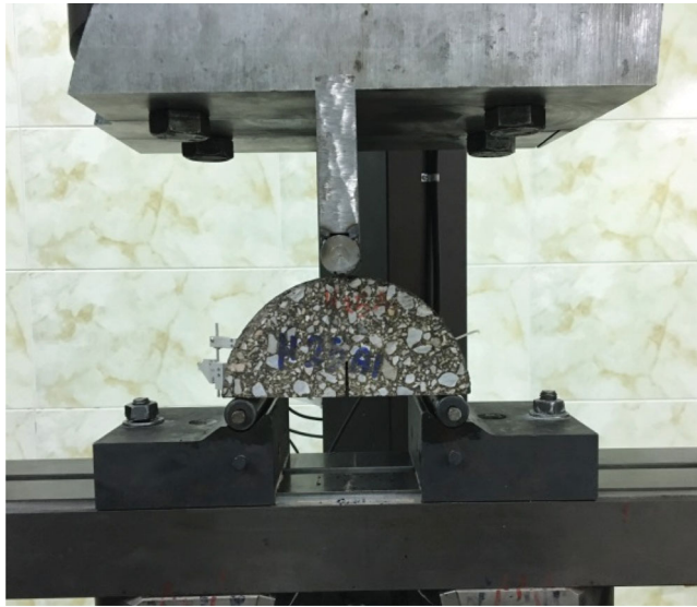
Figure 2. The fixture of the SCB fracture test.
