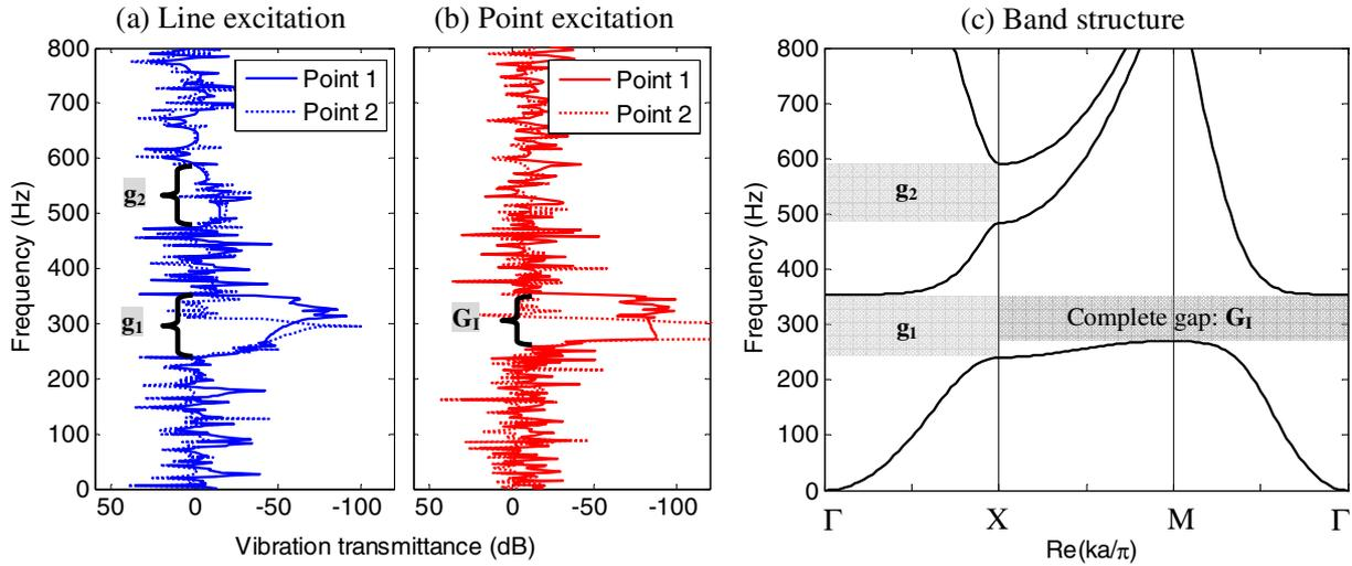
**Figure 7.** Vibration transmittance of the finite LR plate ( $f_R = 300$  Hz) corresponding to the case considered in figure 2(a) under (a) line excitation and (b) point excitation. For ease of comparison, the band structure of the infinite system, which has been shown in figure 2(a), is replotted here in (c). The location and width of the transmission gaps revealed by the solid lines in (a) and (b) are in good agreement with the band gaps shown in (c).
