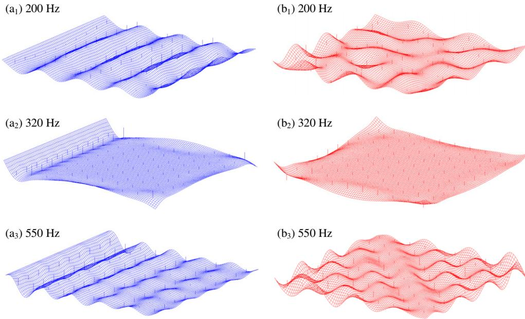
**Figure 8.** Steady-state wave profiles of the finite LR plate considered in figure 7: (a<sub>1</sub>)–(a<sub>3</sub>) line excitation, (b<sub>1</sub>)–(b<sub>3</sub>) point excitation. Note that, at a frequency of 320 Hz (inside the gaps  $g_1$  and  $G_I$ ), the excited waves can propagate without considerable attenuation along the free edges of the finite structure, but are significantly suppressed in the interior area of the structure.
