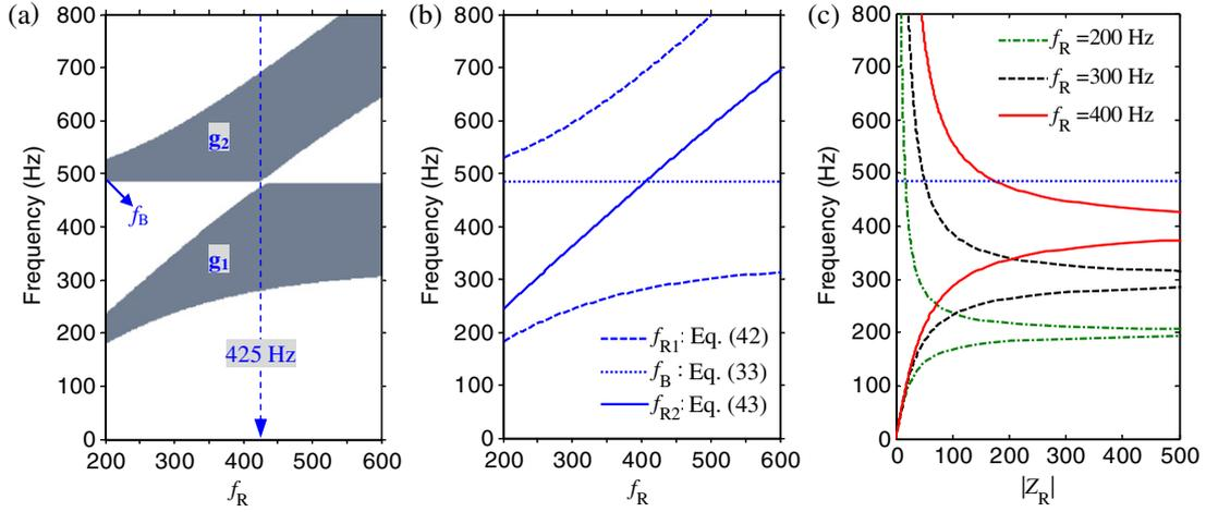
**Figure 3.** (a) Maps of the two directional gaps  $g_1$  and  $g_2$  as a function of the resonant frequency  $f_R$ . The parameters of the plate, the lattice constant and the resonator masses are all fixed, and they are chosen to be the same as in figure 2. (b) Analytically calculated BEFs based on an approximate model of the system considered in (a). (c) Evolution of the magnitude of the mechanical input impedance of the resonators ( $|Z_R|$ ) with increasing resonant frequency  $f_R$ .
