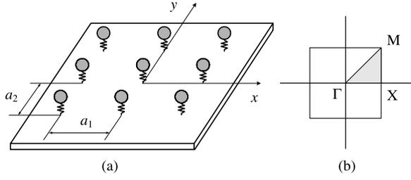
**Figure 1.** (a) Schematic diagram of a LR thin plate with a 2D periodic array of attached spring–mass resonators. (b) Corresponding first Brillouin zone of the periodic lattice. The grey area in (b) is the irreducible region of the Brillouin zone.
