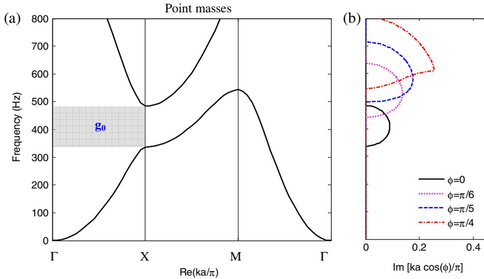
**Figure 5.** Complex band structures for a periodic system made of a thin plate with periodically attached point masses: (a) the real wave band structure, (b) the imaginary part of Bloch wave vectors. The parameters of the plate, the lattice constant and the masses are all the same as in figures 2 and 4. Note that along the  $\Gamma X$  direction only a Bragg gap  $\mathbf{g}_0$  exists. Moreover, no complete band gap is achieved in the system.
