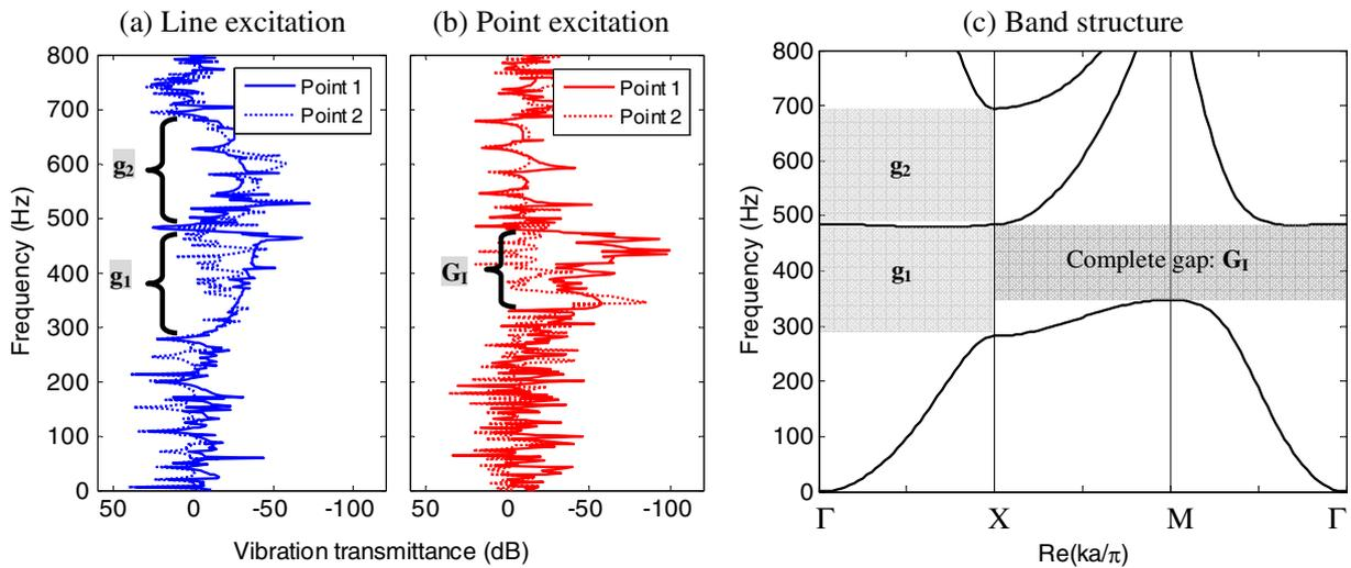
**Figure 9.** The same as in figure 7, but for the finite LR plate ( $f_R = 425$  Hz) corresponding to the case considered in figure 2(b). The regions of the vibration transmission gaps revealed by the solid lines in (a) and (b) match well with the band gaps shown in (c).
