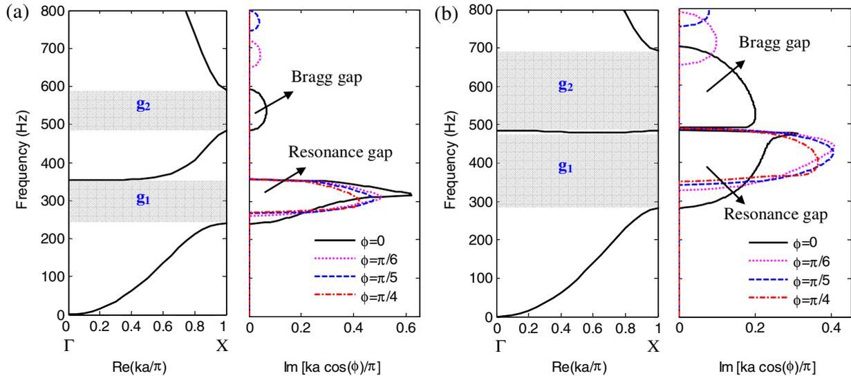
**Figure 4.** Complex band structures calculated by equation (32) for the two LR plate systems considered in figure 2: (a)  $f_R = 300$  Hz, (b)  $f_R = 425$  Hz. In the left panels of (a) and (b), only the solutions along the  $\Gamma X$  direction ( $\phi = 0$ ) are shown, but in the right panels, the solutions along four different directions are depicted for comparison. The case of  $\phi = \pi/4$  represents the  $\Gamma M$  direction.
