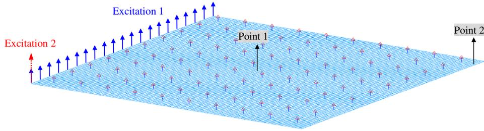
**Figure 6.** Finite element model of a LR plate with  $10 \times 10$  unit cells. ‘Excitation 1/2’ represents a line/point harmonic displacement excitation. The vibration transmittances at points 1 and 2 are calculated.
