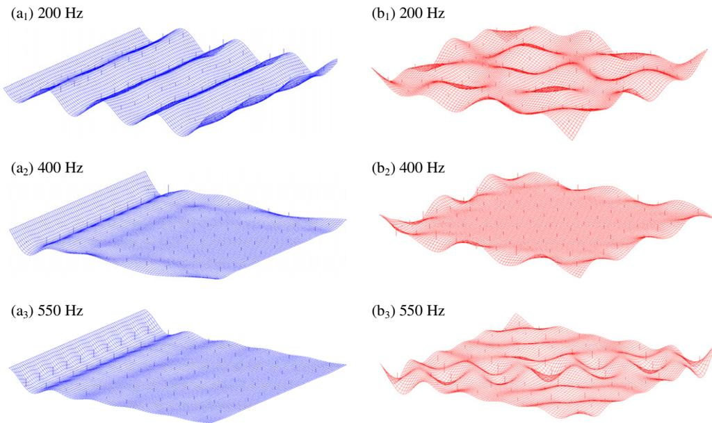
**Figure 10.** Steady-state wave profiles of the finite LR plate—considered in figure 9: (a<sub>1</sub>)–(a<sub>3</sub>) line excitation, (b<sub>1</sub>)–(b<sub>3</sub>) point excitation. Note that, at the frequency 400 Hz, the excited waves can propagate along the free structure edges more easily than through the interior area of the structure, as shown in (a<sub>2</sub>) and (b<sub>2</sub>).
